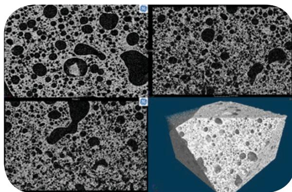
Processing of images to enable quantification of voids – includes 3D reconstruction
