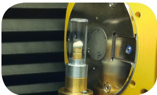
A sample of ice cream mounted in a  $\mu$ XCT system
